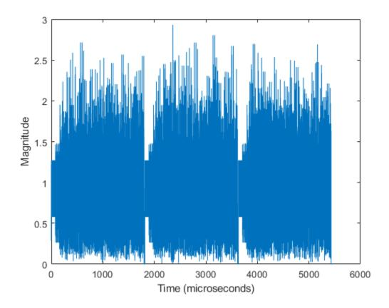
The plot shows three S1G format packets, with each packet separated by 15 microseconds of idle time.
