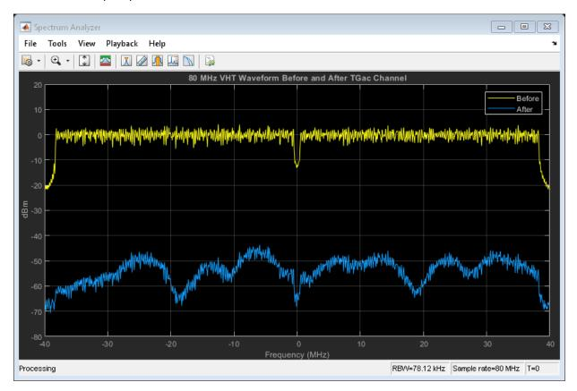
Path loss accounts for the roughly 50 to 60 dB of separation between the waveform before and after it passes through the TGac channel. The path loss results from the default transmitter-to-receiver distance of 3 meters, and from shadowing effects. The signal level variation shows the frequency selectivity of the delay profile across the frequency spectrum.
