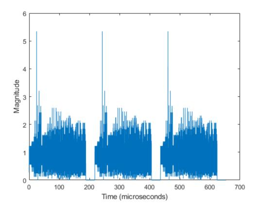
The plot shows three multiuser HE format packets, with each packet separated by 30 microseconds of idle time.
